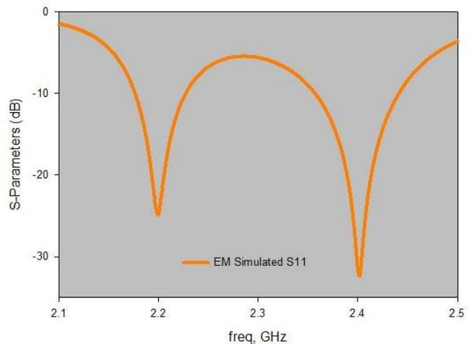
Fig. 11. Input port reflection responses of diplexer full-wave simulation
