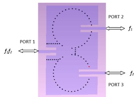
Fig. 1: Operation principle of the proposed SIW diplexer.
