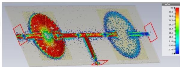
Fig. 14. The diplexer surface current distribution in the cavity at 2.4 GHz.
