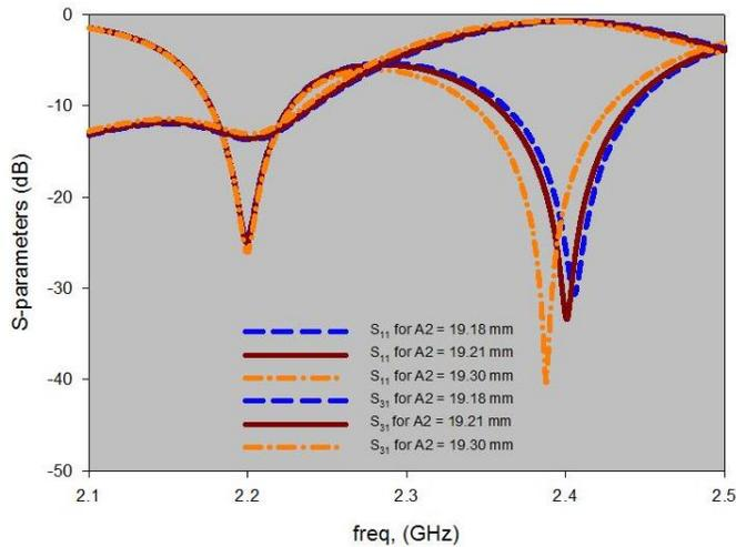
Fig. 8: Simulated  $|S_{11}|$  and  $|S_{31}|$  for the 2.4 GHz SIW cavity with different  $A2$
