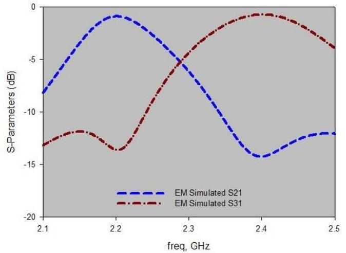
Fig. 9. Transmission responses of diplexer full-wave simulation
