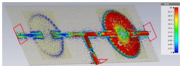
Fig. 13. The diplexer surface current distribution in the cavity at 2.2 GHz.
