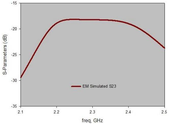
Fig. 10. Isolation between output ports of diplexer full-wave simulation
