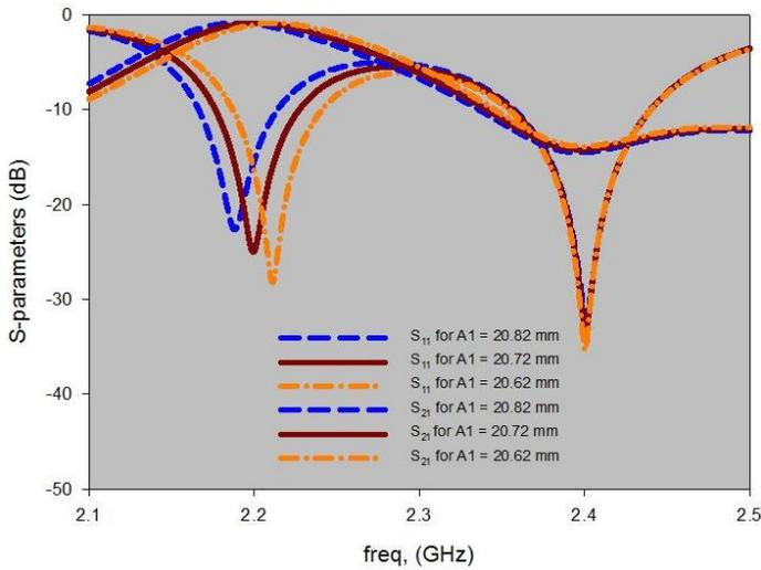
Fig. 7: Simulated  $|S_{11}|$  and  $|S_{21}|$  for the 2.2 GHz SIW cavity with different  $A1$
