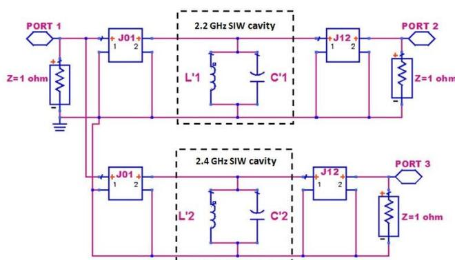
Fig. 2: Lumped element equivalent circuit for the diplexer
