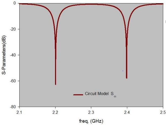
Fig. 5: Circuit model input port reflection
