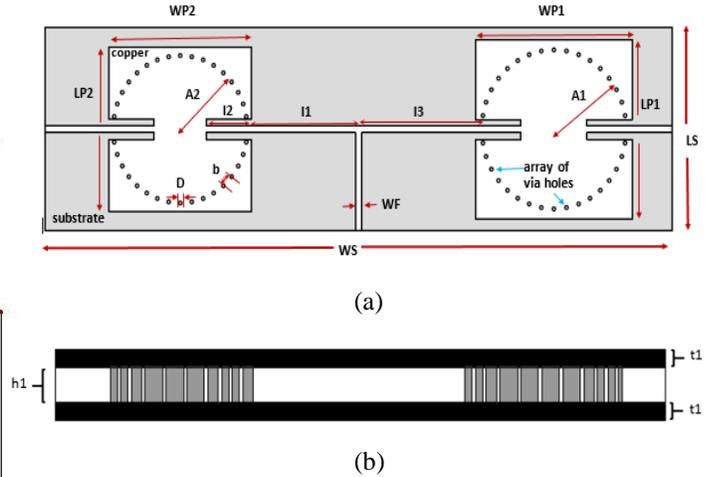
Fig. 6: Configuration of the First-order SIW diplexer (a) top view, (b) side view.
