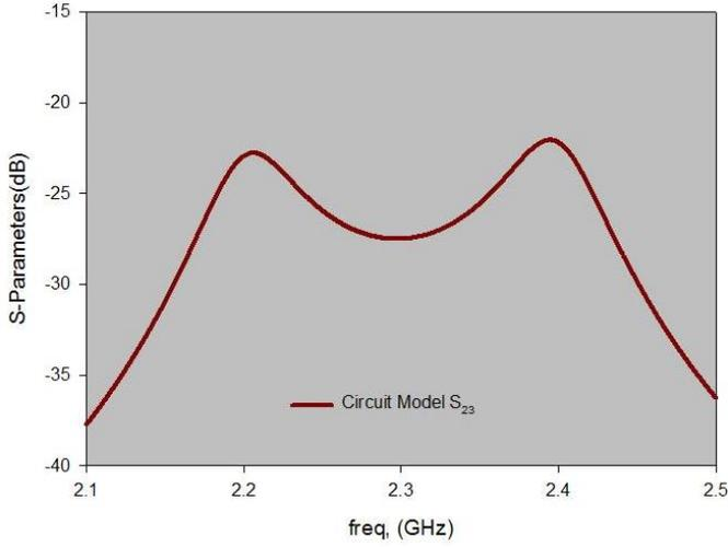
Fig. 4: Circuit model isolation between output ports
