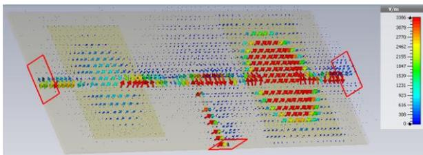
Fig. 12. The diplexer E-field distribution in the cavity at 2.2 GHz.
