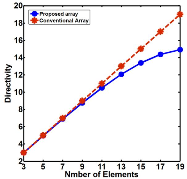
Fig. 5. Directivity as a function of the number of array elements
