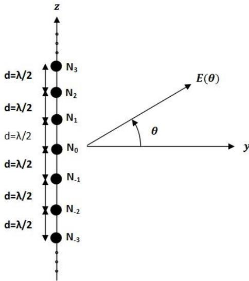
Fig. 2. Symmetric phased array antenna arrangement by moving phase reference to the centre element.
