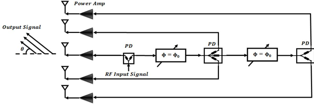
Fig. 3. Proposed phased array transmitter
