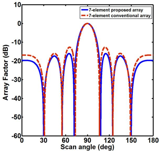
Fig. 4. Normalized array factor for a 7-element linear phased array
