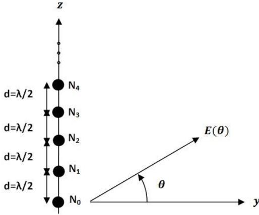
Fig. 1. An N-elements conventional phased array antenna
