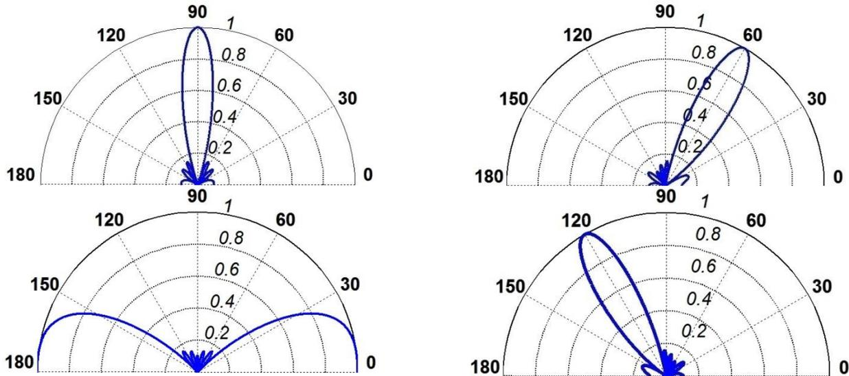
Fig. 6. Array patterns of the 7-element proposed phased array system. The antenna spacing is assumed to be half wavelength
