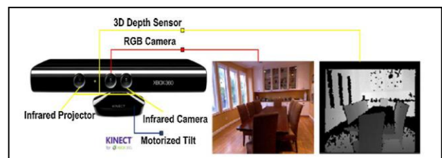
Figure 1 : Hardware configuration of Kinect and images captured by RGB camera and depth sensor [5]
