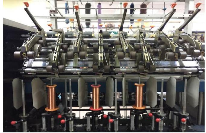
Fig. 2. Hollow spindle machine YCHN-303 used in constructing conductive threads
