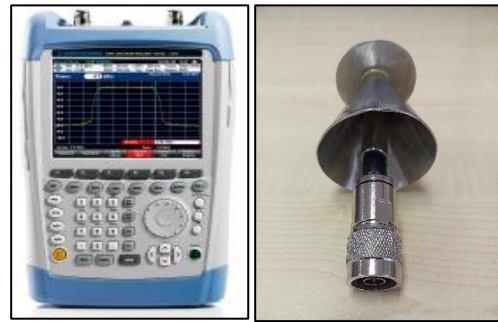
Fig. 1. The instruments used for the RFI scanning: Spectrum analyzer (left-hand-side); Multiband discone antenna (right-hand-side).
