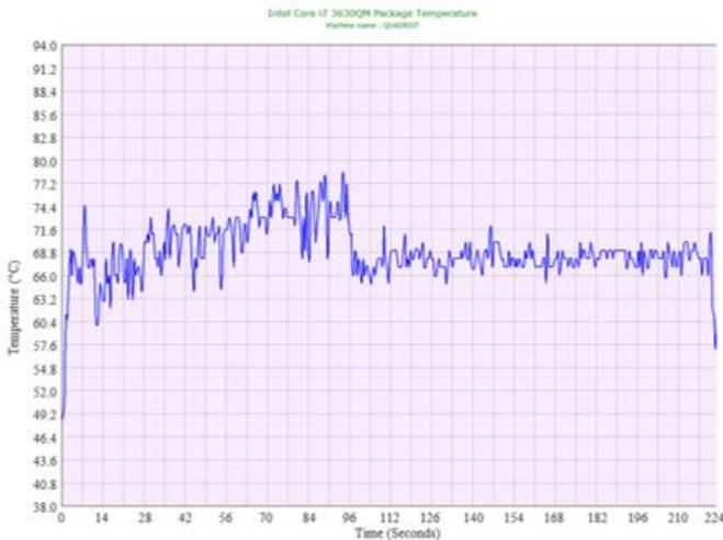
Figure 7: Temperature versus time of stress tests using cooling pad
