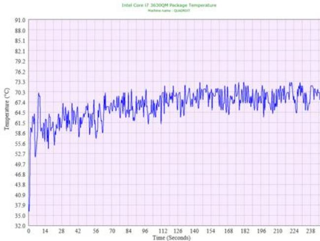
Figure 6: Temperature versus time of stress test using cooled air cooling system
