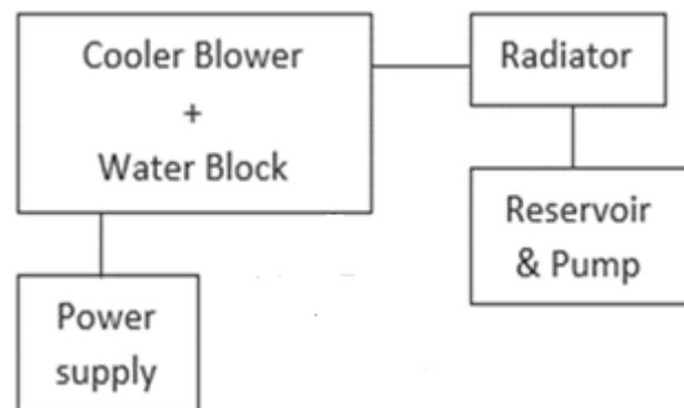
Figure 1: Cooling System Block Diagram
