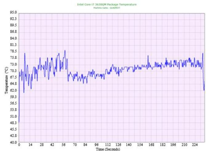
Figure 8: Temperature versus time of stress test using stock cooling system
