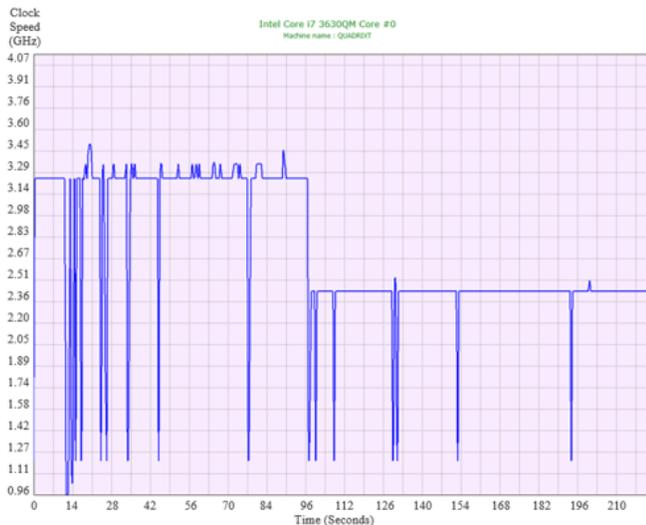
Figure 10: Clock speed versus time of stress test using cooled air cooling system. The CPU clock speed maintains at 3.2 GHz for 98 seconds then drop to 2.4 GHz until end of test
