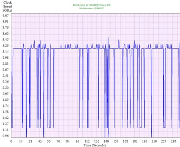
Figure 9: Clock speed versus time of stress test using cooled air cooling system. The CPU clock speed maintain at 3.2GHz for entire test time
