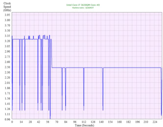
Figure 11: Clock speed versus time of stress test using cooled air cooling system. The CPU clock speed maintains at 3.2 GHz for 63 seconds and drop to 2.4 GHz until end of test.
