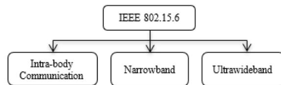
Fig.1. Physical Layers of IEEE 802.15.6 standard
