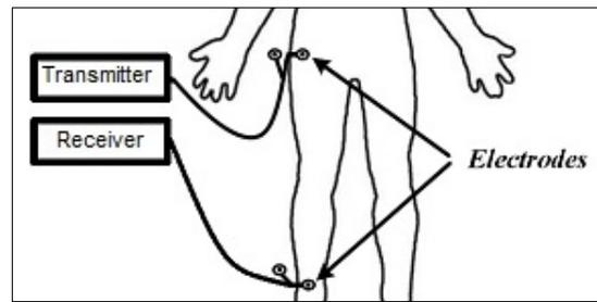
Fig. 7. Capacitive coupling IBC setup
