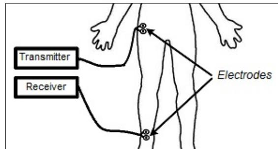
Fig. 6. Galvanic coupling IBC setup
