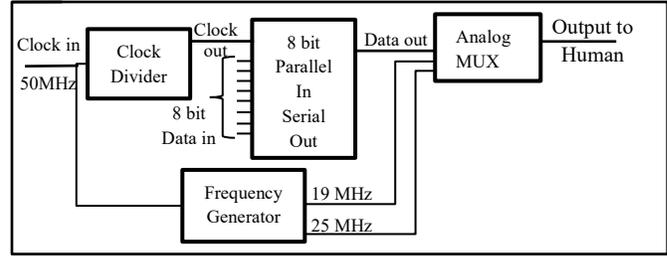
Fig. 8. Block Diagram BFSK Transmitter
