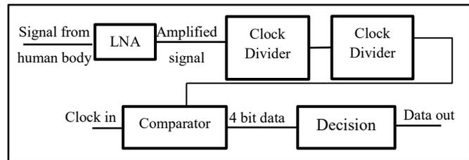
Fig. 9. Block Diagram of BFSK Receiver
