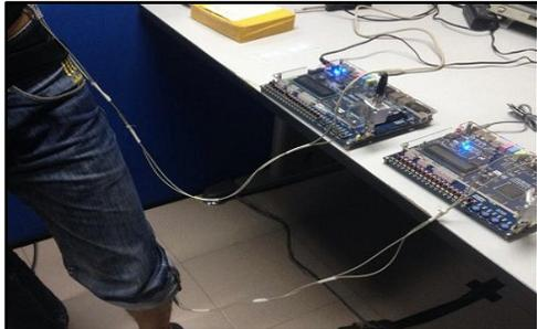
Fig. 11. IBC Transceiver measurement setup
