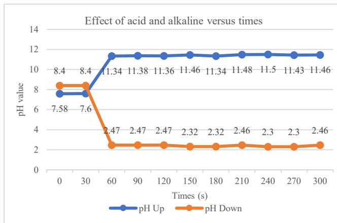
Fig. 3. Water pH value for both acid and alkaline case versus time
