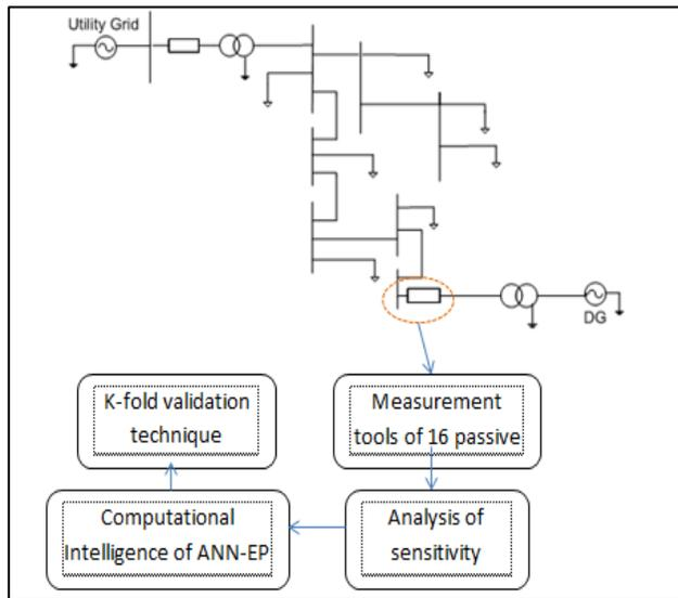
Fig. 1 Concept of the proposed islanding detection technique
