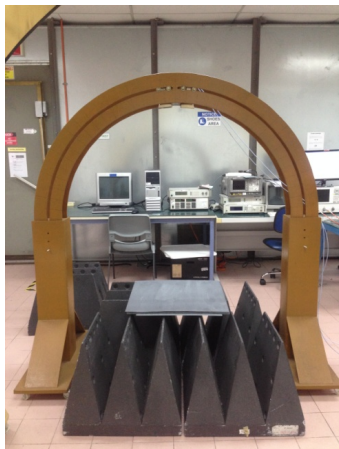
Fig. 3. Measurement set up by using NRL arch free space method
