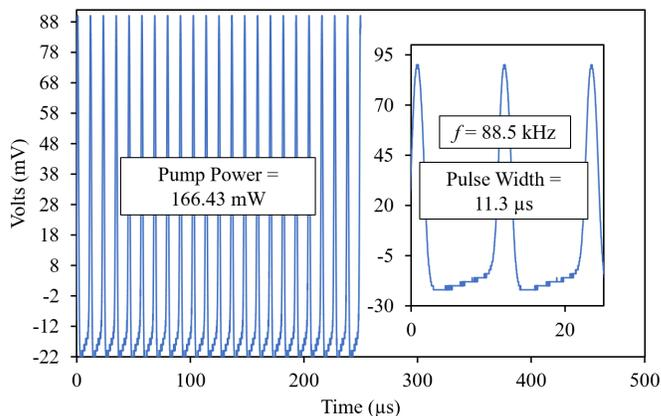
Fig. 10. Stability of pulse train at a pump power of 166.43 mW
