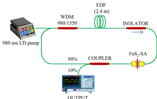
Fig. 6. Ring cavity setup of the EDFL Q-switched.
