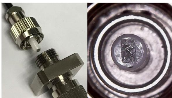
Fig. 7. FeS<sub>2</sub> film on fiber ferrule.
