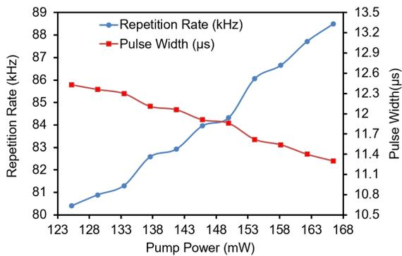
Fig. 11. Repetition rate and pulse width of the input laser.
