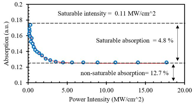
Fig. 5. Nonlinear optical profile of FeS<sub>2</sub>-SA.
