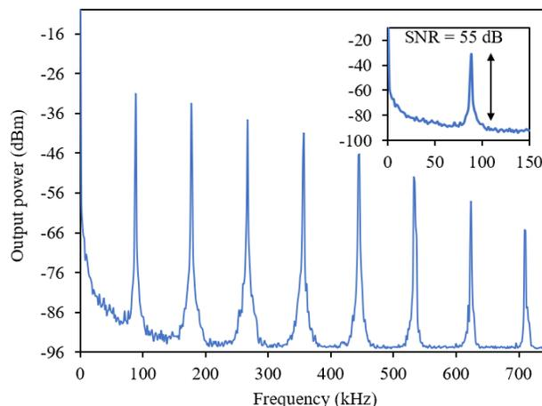
Fig. 9. RF spectrum at 166.43 mW of pump power.
