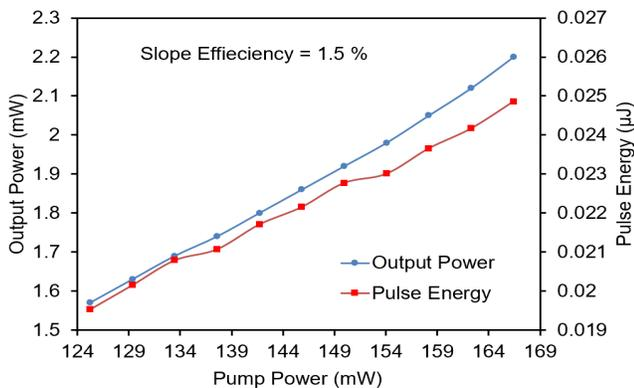
Fig. 12. Average power and peak pulse power of the input laser versus pump power.
