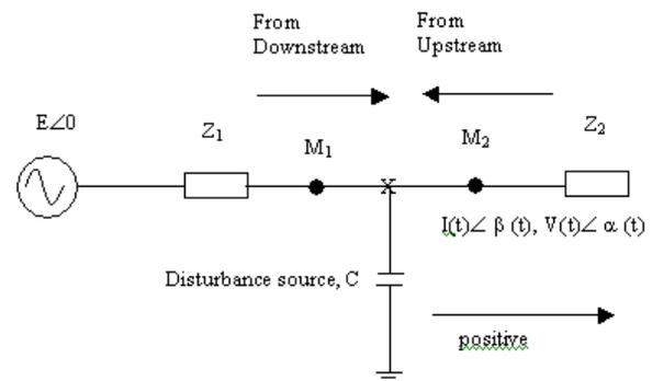
Fig. 2. Illustrating the transient source location analysis
