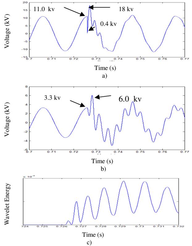
Fig. 7 Magnification of capacitor voltage at MTG a) Transient Voltage b) Magnifying Voltage c) Wavelet Energy
