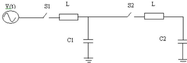
Fig. 1. Simplified circuit with L-C loops
