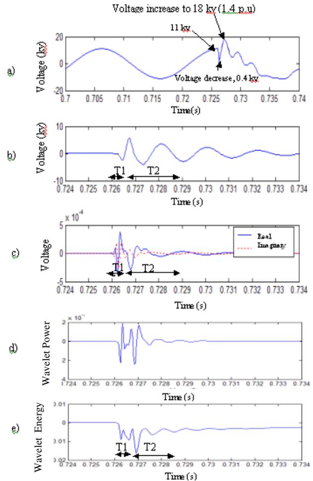
Fig. 4 Results from normal capacitor switching at PCC a) Original Voltage b) Filtered Voltage c) Complex Wavelet Voltage d) Complex Wavelet Power e) Complex Wavelet Energy
