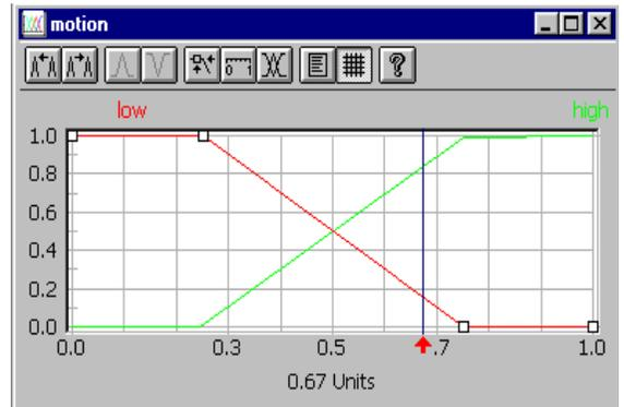
Fig. 5: The Fuzzy Input Variable 'Motion'
