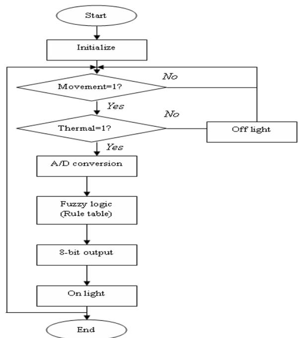
**Fig. 2:** Flow Chart of Intelligent Lighting Control System
