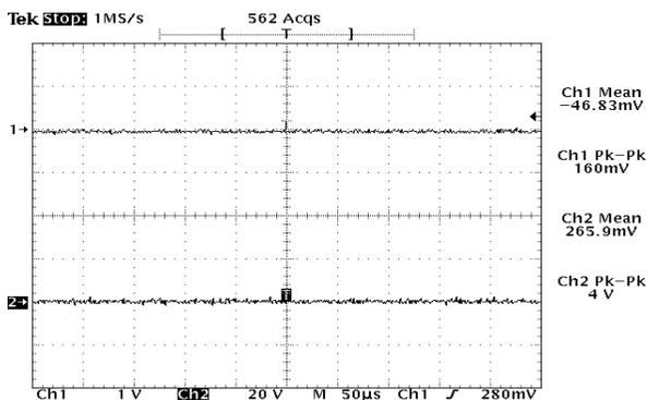
Fig.7: Waveform of the Output Sensor for No Human Presence
