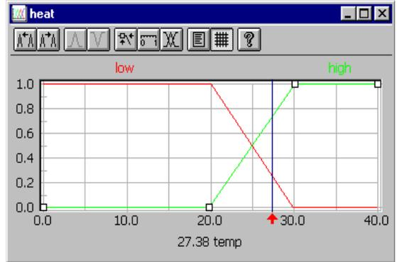
FIG. 4: The Fuzzy Input Variable 'Heat'
