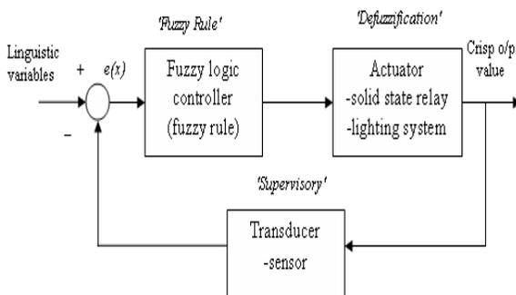
**Fig. 1:** Block Diagram of Fuzzy Control System
