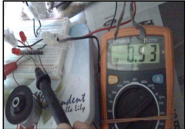
Figure 8: Output Voltage from TEG module
