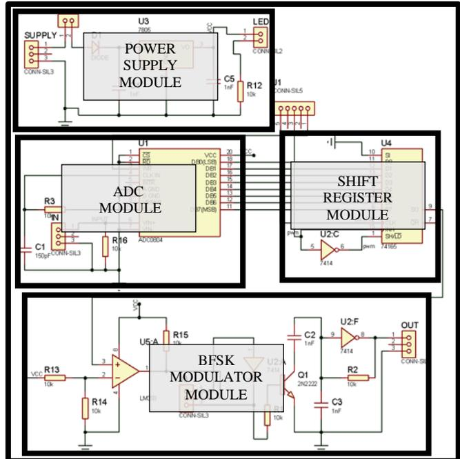
Figure 2.6: Implementation of transmitter module
