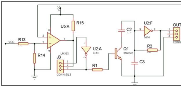
Figure 2.5: BFSK modulator module setup
