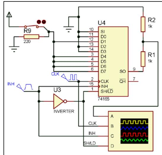
Figure 2.3: Shift register module setup
