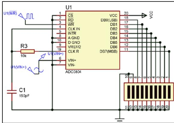
Figure 2.2: ADC module setup
