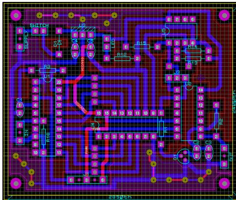
Figure 2.8: PCB layout for transmitter module
