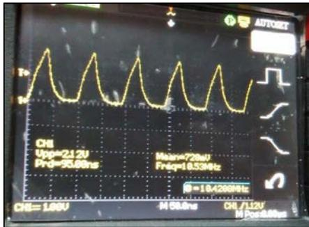
Figure 3.5: 10.4MHz frequency produced at high input signal
