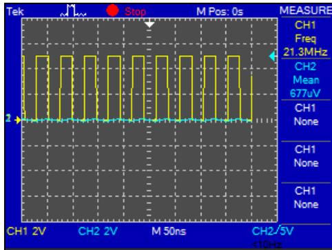
Figure 3.4: 21.3MHz frequency produced at low signal input
