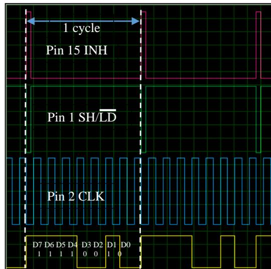
Figure 3.2: Waveform data output
