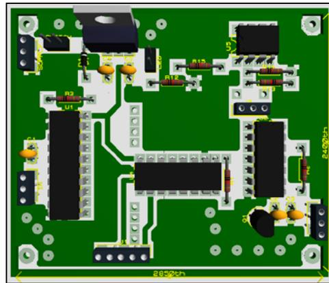
Figure 2.7: Transmitter module circuit layout
