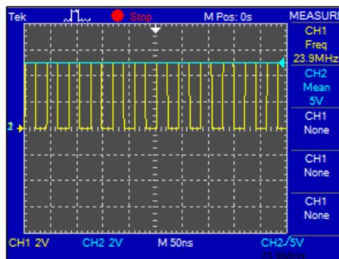
Figure 3.3: 23.9MHz frequency produced at high signal input
