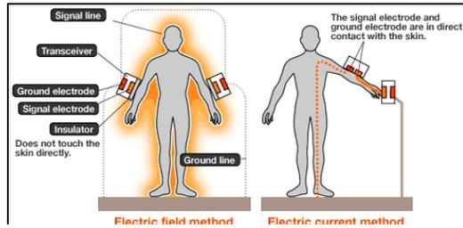
Figure 1.1: Example of measurement setup of IBC
