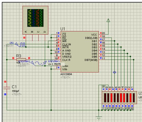
Figure 3.1: ADC design circuit diagram and output data
