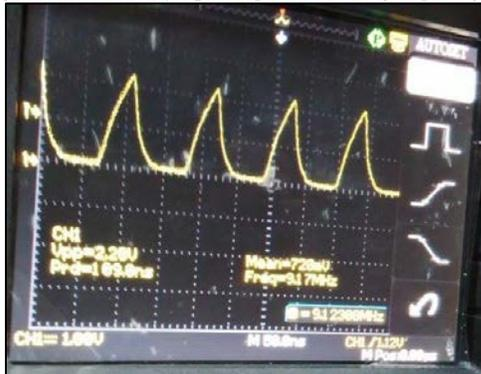
Figure 3.6: 9.1MHz frequency produced at low input signal
