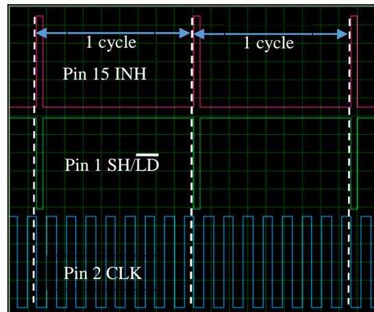
Figure 2.4: Clock setup for shift register
