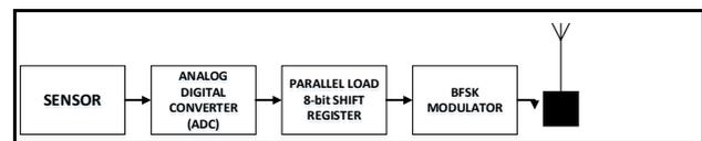
Figure 2.1: Block diagram transmitter module using off-the-shelf component
