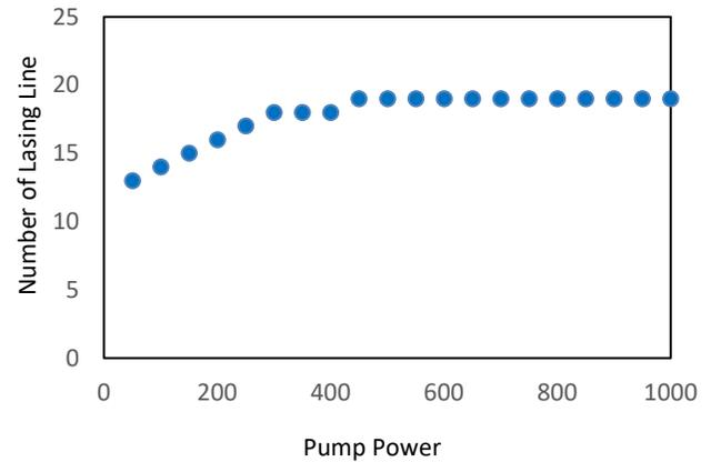
Fig. 9. Number of lasing line versus pump power for bidirectional linear laser.
