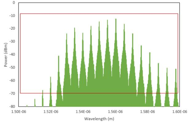
Fig. 12. Multiwavelength output signal from ring laser with 50% arm of an optical coupler (OC).
