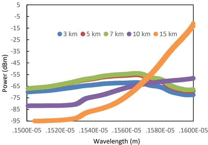
Fig. 5. Raman Amplifier (FRA) gain with different length.
