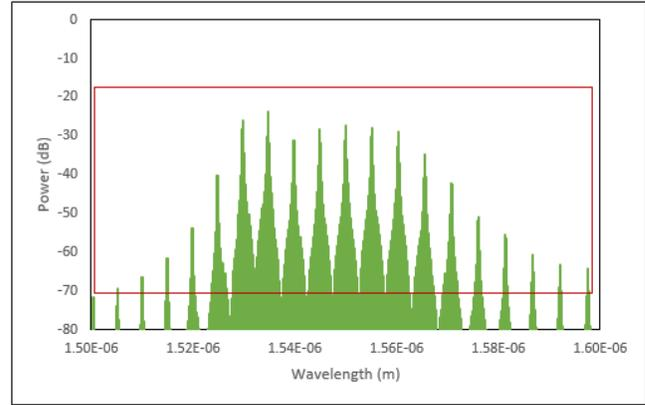
Fig. 8. Multiwavelength output signal from single pass linear laser with 50% arm of an optical coupler (OC).
