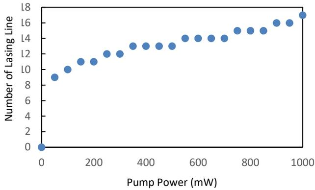
Fig. 7. Number of lasing line versus pump power for single pass linear laser.
