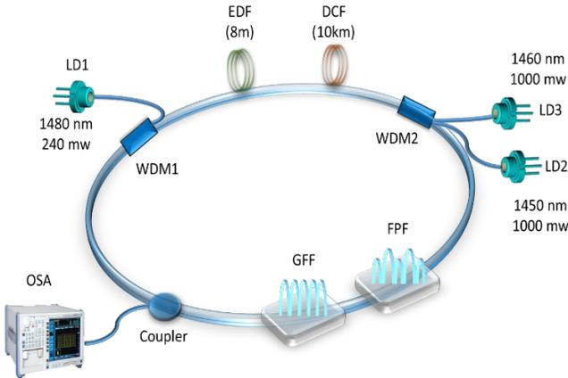
Fig. 3. Schematic configuration of the multiwavelength ring cavity laser.
