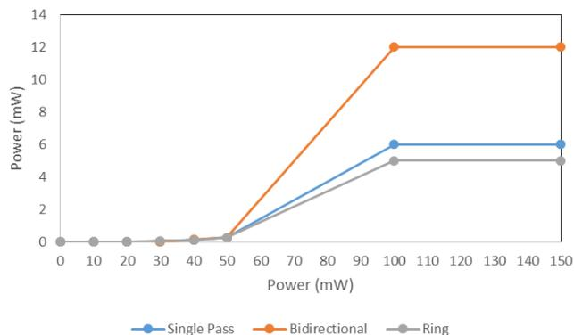
Fig. 13. Total pump power versus Total output power.
