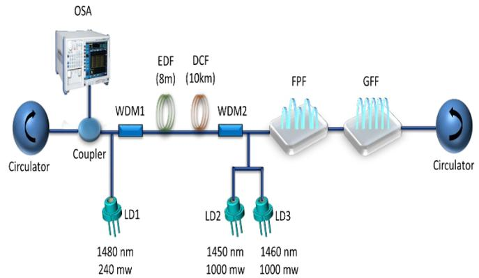
Fig. 1. Schematic configuration of the multiwavelength single pass linear cavity laser.
