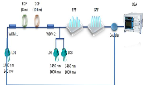
Fig. 2. Schematic configuration of the multiwavelength bidirectional linear cavity laser.
