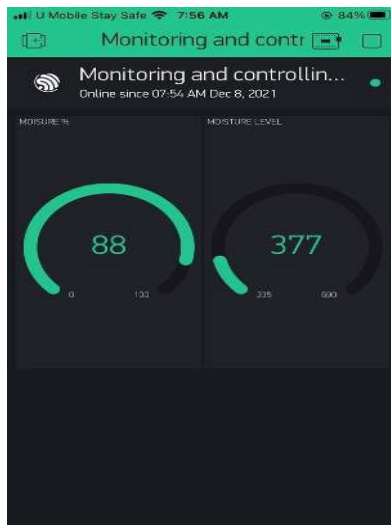
Fig. 7. Blynk interface for moisture level and its percentage for moisture condition below than 500.
