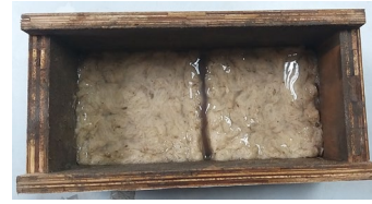
Fig. 2. PALF-PDMS mixture spread in mold
